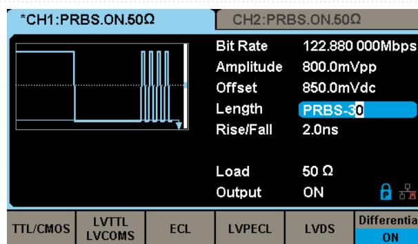
Preset common logic levels such as TTL, LVCMS, LVPECL and LVDS. An added differential mode provides an easy way to generate differential signals using the both channels.
