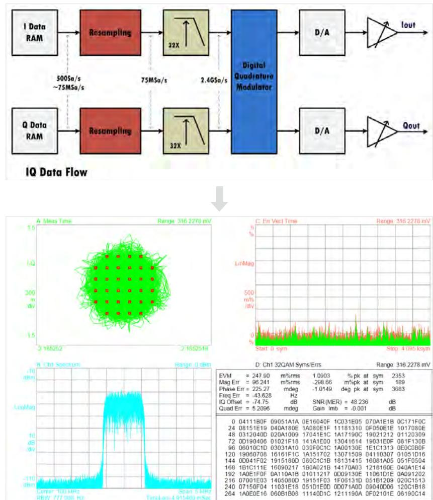
The SDG6000X supports popular modulation types such as ASK, FSK, PSK, and QAM. Proprietary resampling technology provides excellent EVM performance at arbitrary symbol rates between 250 Symb/s ~ 37.5 MSymb/s. Built-in digital quadrature modulator provides the possibility to generate IQ signals from baseband to 500 MHz intermediate frequency.
