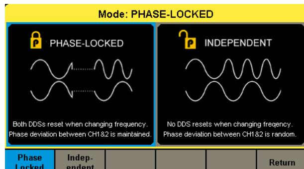
"Phase-Locked" mode automatically aligns the phases of each output. While "Independent" mode permit the two channels to be used as two independent generators. Independent mode also smoothes parameter (frequency, amplitude) changes made to an active channel.
