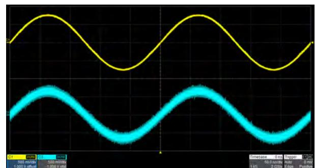
Wideband Gaussian noise can be easily added to other waveforms to simulate real-world scenarios in which the signal contains a large degree of noise.
