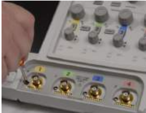
Figure 21 Removing the T6 screws
