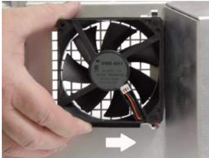
Figure 35 Removing fan assembly
