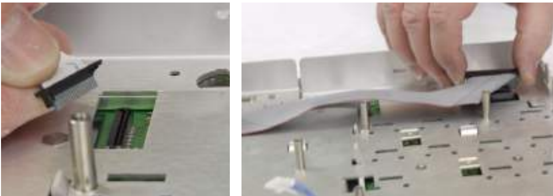
Figure 26 Removing keyboard cables
