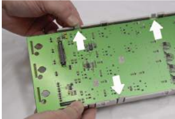
Figure 32 Separating front panel from printed circuit board
