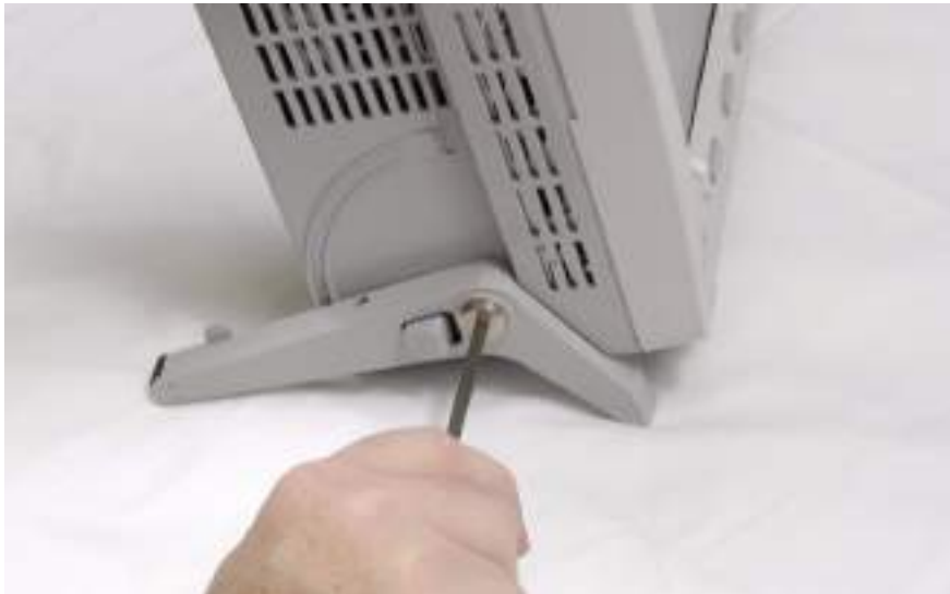
Figure 17 Removing adjustable leg
