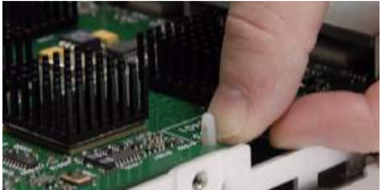
Figure 23 Unlocking alignment pin
