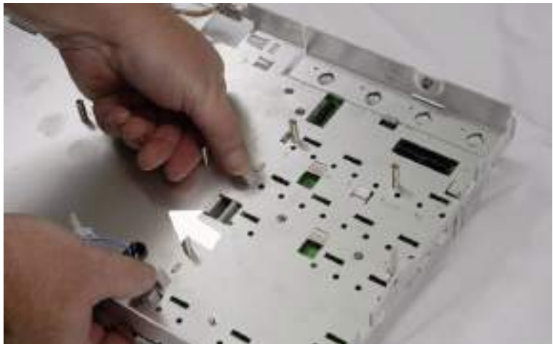
Figure 30 Removing front panel assembly from front deck
