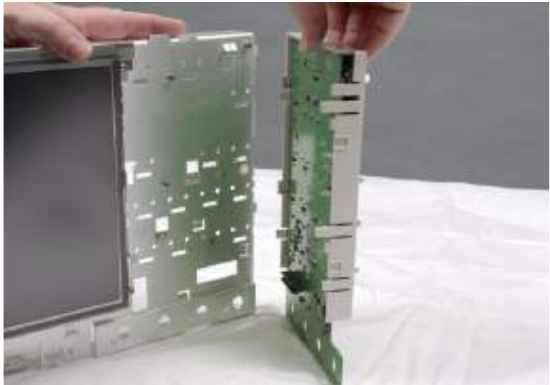
Figure 30 Removing front panel assembly from front deck
