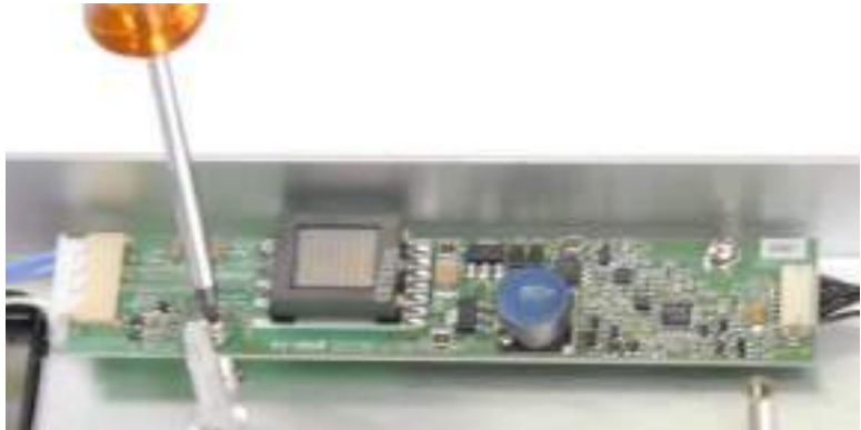
Figure 24 Removal of inverter board
