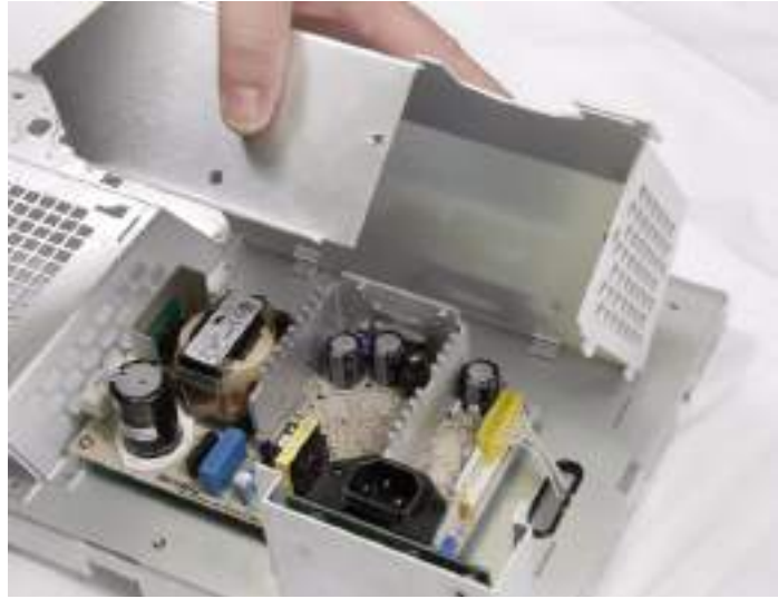
Figure 37 Lifting power supply cover off
