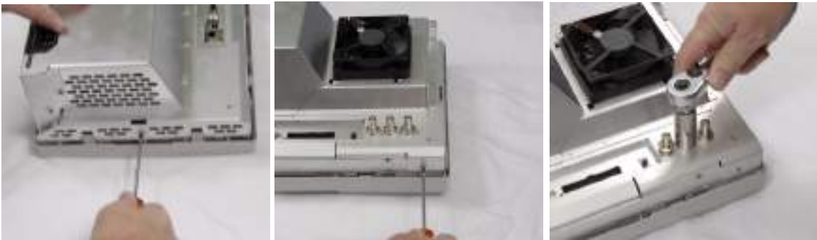
Figure 19 Removing the rear deck assembly
