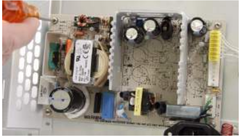
Figure 38 Removing the power supply
