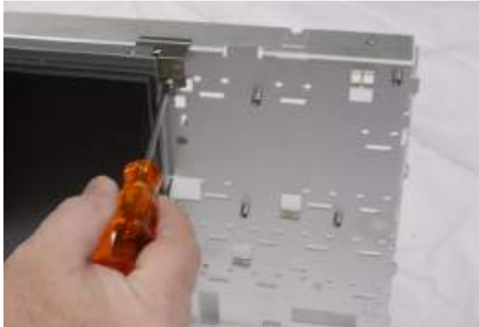
Figure 34 Removing display assembly
